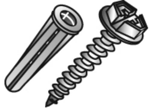
*An injection-molded anchor with a flanged opening at the top end and a cone-shaped body that is cupped at the opposite end.*
